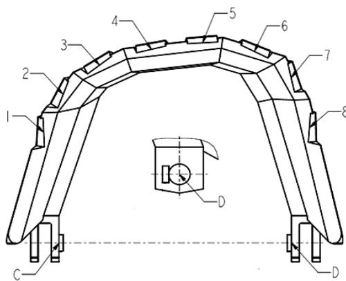
**Fig.8.** Measure points of blade geometry verification
