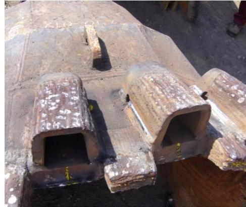
**Fig. 7.** Failure of teeth
