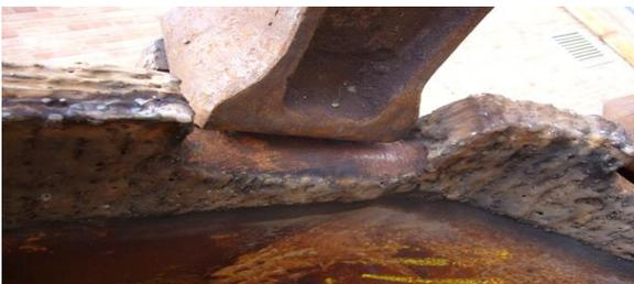
**Fig. 3.** The deficiency of the relative position of the tooth on cutting blade at the renewed buckets
