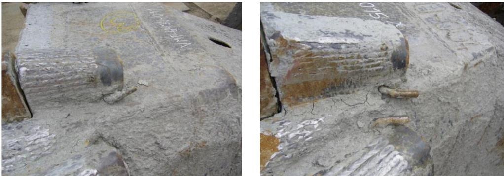
**Fig. 4-5.** Wrong positioning of the tooth adapters on the renewed buckets
