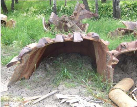
**Fig. 6.** Renewed cutting blade with adapters
